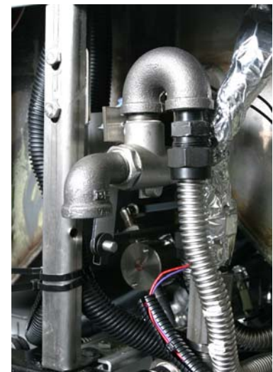
Figure 4: The oil disposal valve is shown attached to the upright. The down pipe has been removed to ease replacement of the fryer back.
