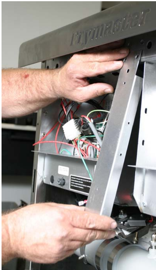
Figure 6: Remove the panel between the control boxes and above the filter pan.
